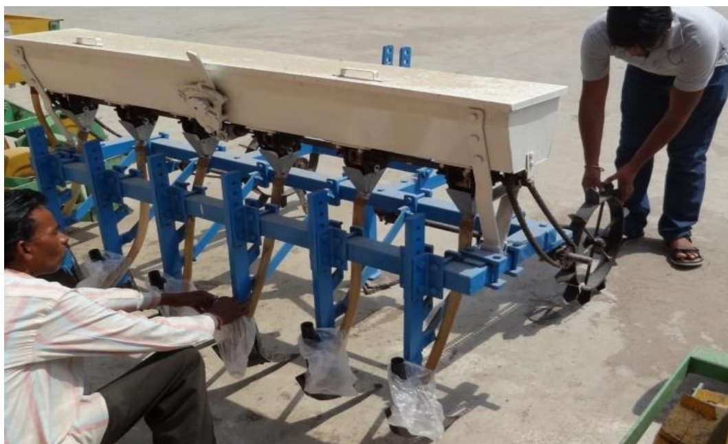
Fig. 1: Calibration of fertilizer applicator in the laboratory
