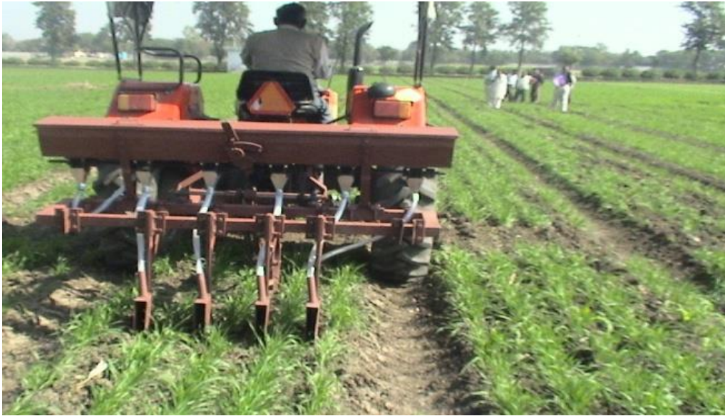
Fig. 2: Field testing of the fertilizer applicator on the wheat crop (21 days).
