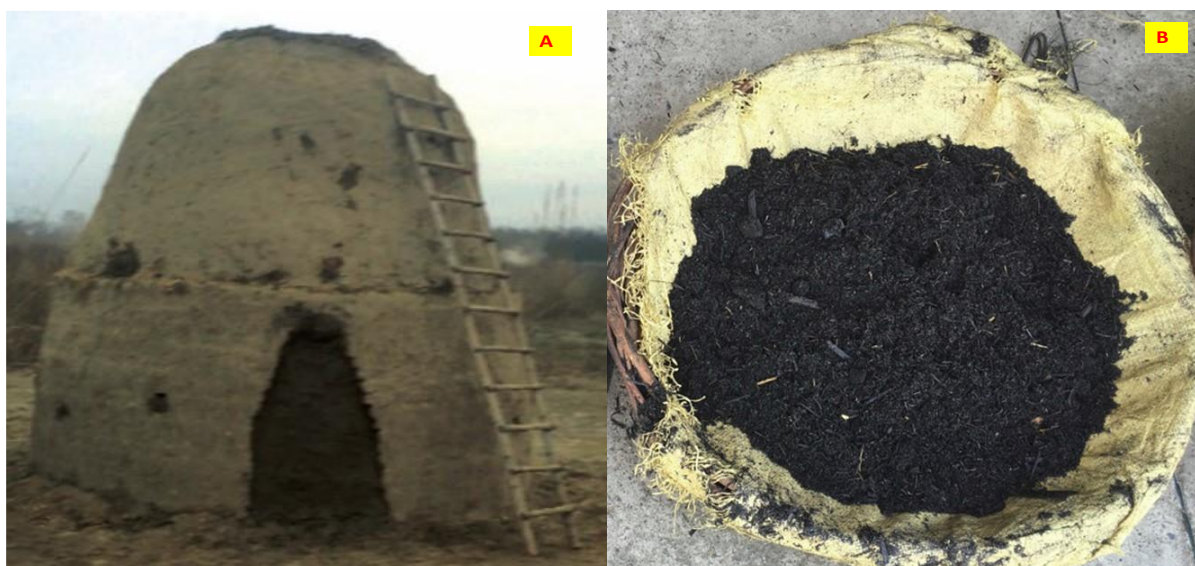
Fig. 1 Preparation of paddy straw biochar (A) Kiln for preparing paralichar (B) Paralichar.
