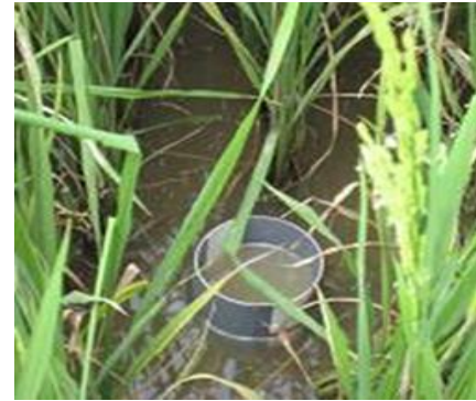
Perforated PVC pipe to examine the below-ground water table in AWD
