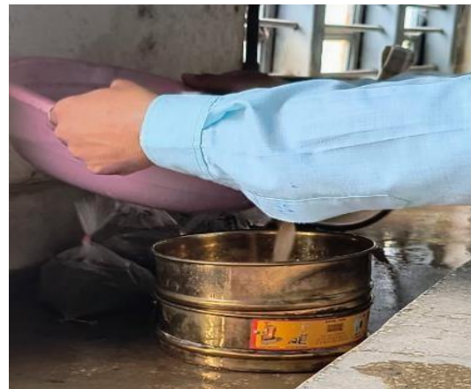
Fig. 2. Sample wash with water using 25 and 325 mesh sieves.
