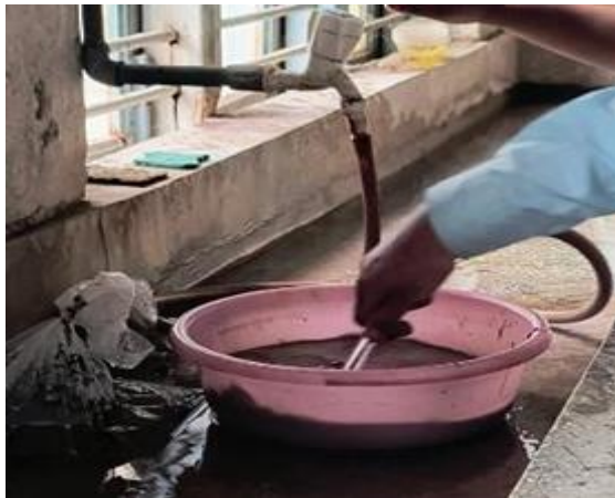
Fig. 2. Sample wash with water using 25 and 325 mesh sieves.
